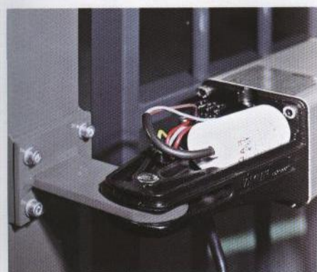
Detail of capacitor fixed into place
